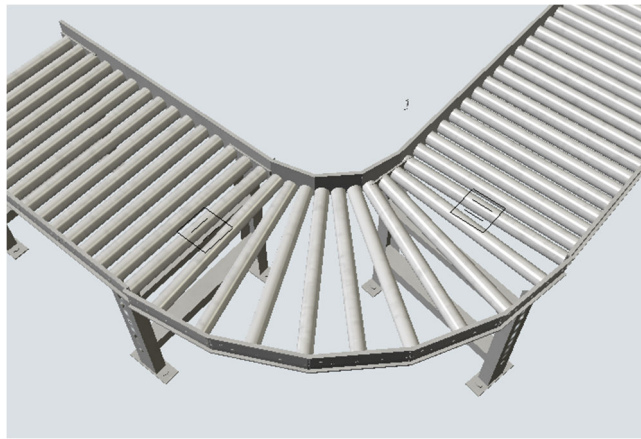
Fig. 8 Connecting conveyors using Join Conveyors
