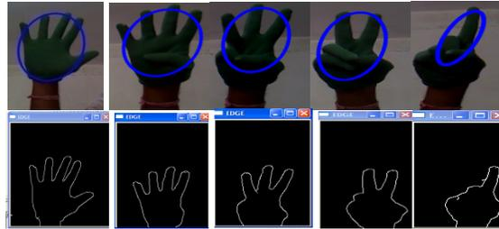
**FIGURE 5:** Segmentation results on green color glove
