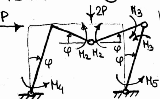
$$\left. \begin{aligned} L_{ext} &= 2P \varphi \frac{L}{2} + P \varphi L = 2P \varphi L \\ L_{int} &= 2M_2 \varphi + 2M_3 \varphi + M_4 \varphi + M_5 \varphi \end{aligned} \right\} P_{II} = \frac{M_2}{4} + \frac{M_3}{4} + \frac{M_4}{8} + \frac{M_5}{8} \text{ [kN]}$$
