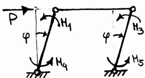
$$\left. \begin{aligned} L_{ext} &= P \varphi L \\ L_{int} &= M_1 \varphi + M_3 \varphi + M_4 \varphi + M_5 \varphi \end{aligned} \right\} P_{III} = \frac{M_1}{4} + \frac{M_3}{4} + \frac{M_4}{4} + \frac{M_5}{4} \text{ [kN]}$$
