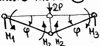
$$\left. \begin{aligned} L_{ext} &= 2P \cdot \varphi \cdot \frac{L}{2} = P \cdot \varphi \cdot L \\ L_{int} &= M_1 \varphi + 2M_2 \varphi + M_3 \varphi \end{aligned} \right\} P_I = \frac{M_1}{4} + \frac{M_2}{2} + \frac{M_3}{4} \text{ [kN]}$$
