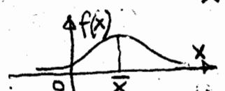
$\sigma_x = \sqrt{\text{Var}(x)}$ ; coefficient of variation  $\gamma_x = \frac{\sigma_x}{\bar{x}}$
