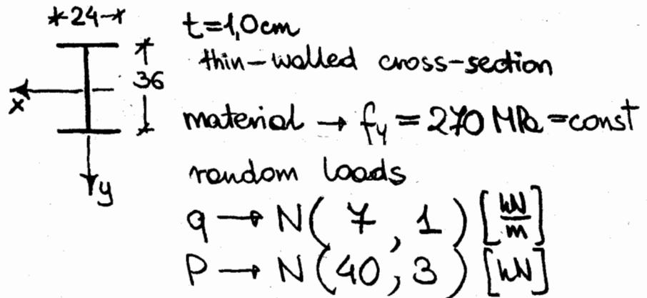
Estimate the probability of the ultimate limit state of the structure, consider bending-compression interaction
