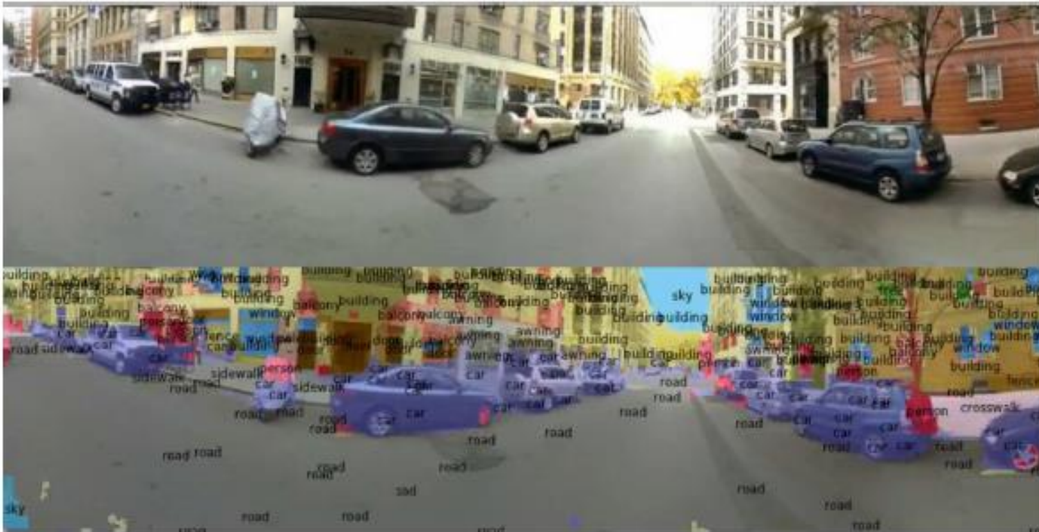
Fig. 11. Real-time scene parsing in natural conditions. Training on SiftFlow dataset. We display one label per component in the final prediction.
