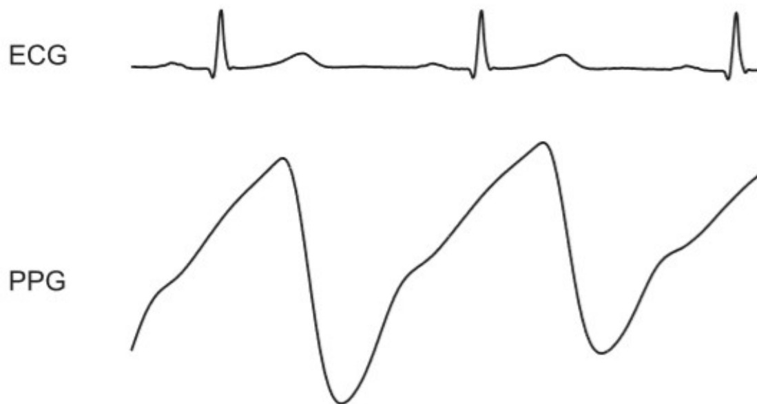
Figure 1. The pulsatile (AC) component of the PPG signal and corresponding electrocardiogram (ECG). The AC component is actually superimposed on a much larger quasi-DC component that relates to the tissues and to the average blood volume within the sample. It represents the increased light attenuation associated with the increase in microvascular blood volume with each heartbeat. In practice, the PPG waveform is often inverted.
