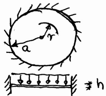
$$W(r) = \frac{qr^4}{64D} + C_1 r^2 + C_2 \quad ; \quad W_{,r} = \frac{qr^3}{16D} + 2C_1 r$$
