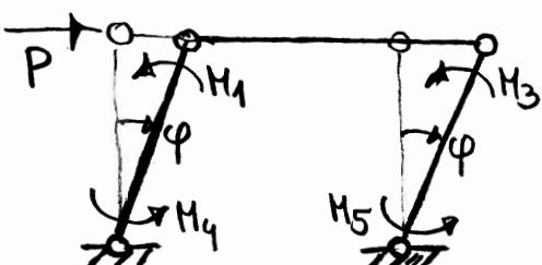
$$\left. \begin{aligned} L_W &= M_1 \varphi + M_3 \varphi + M_4 \varphi + M_5 \varphi \\ L_2 &= P \varphi L \end{aligned} \right\} P_{III} = \frac{M_1}{4} + \frac{M_3}{4} + \frac{M_4}{4} + \frac{M_5}{4} \quad [\text{kN}]$$
