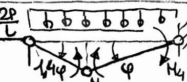
$$\left. \begin{aligned} L_2 &= \frac{2P}{L} \cdot L \cdot \frac{1}{2} \cdot \frac{1}{12} \varphi L = \frac{1}{12} P \varphi L \\ L_W &= 2,4H_3 \varphi + H_4 \varphi \end{aligned} \right\} \quad P_{II} = \frac{36}{35} M_3 + \frac{3}{7} M_4 \quad [\text{kN}]$$
