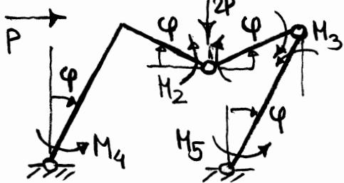
$$\left. \begin{aligned} L_W &= 2M_2 \varphi + 2M_3 \varphi + M_4 \varphi + M_5 \varphi \\ L_2 &= 2P \varphi \frac{L}{2} + P \varphi L = 2P \varphi L \end{aligned} \right\} P_{II} = \frac{M_2}{4} + \frac{M_3}{4} + \frac{M_4}{8} + \frac{M_5}{8} \quad [\text{kN}]$$
