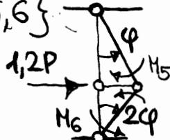
$$\left. \begin{aligned} L_2 &= 1,2P \cdot \frac{2}{3} \varphi L = 0,8P \varphi L \\ L_W &= 3H_5 \varphi + 2H_6 \varphi \end{aligned} \right\} \quad P_{III} = \frac{15}{16} M_5 + \frac{5}{8} M_6 \quad [\text{kN}]$$
