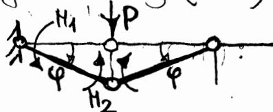
$$\left. \begin{aligned} L_2 &= P \cdot \varphi \cdot \frac{L}{2} \\ L_W &= H_1 \varphi + 2H_2 \varphi \end{aligned} \right\} \quad P_I = \frac{2H_1}{L} + \frac{4H_2}{L} = \frac{H_1}{2} + M_2 \quad [\text{kN}]$$
