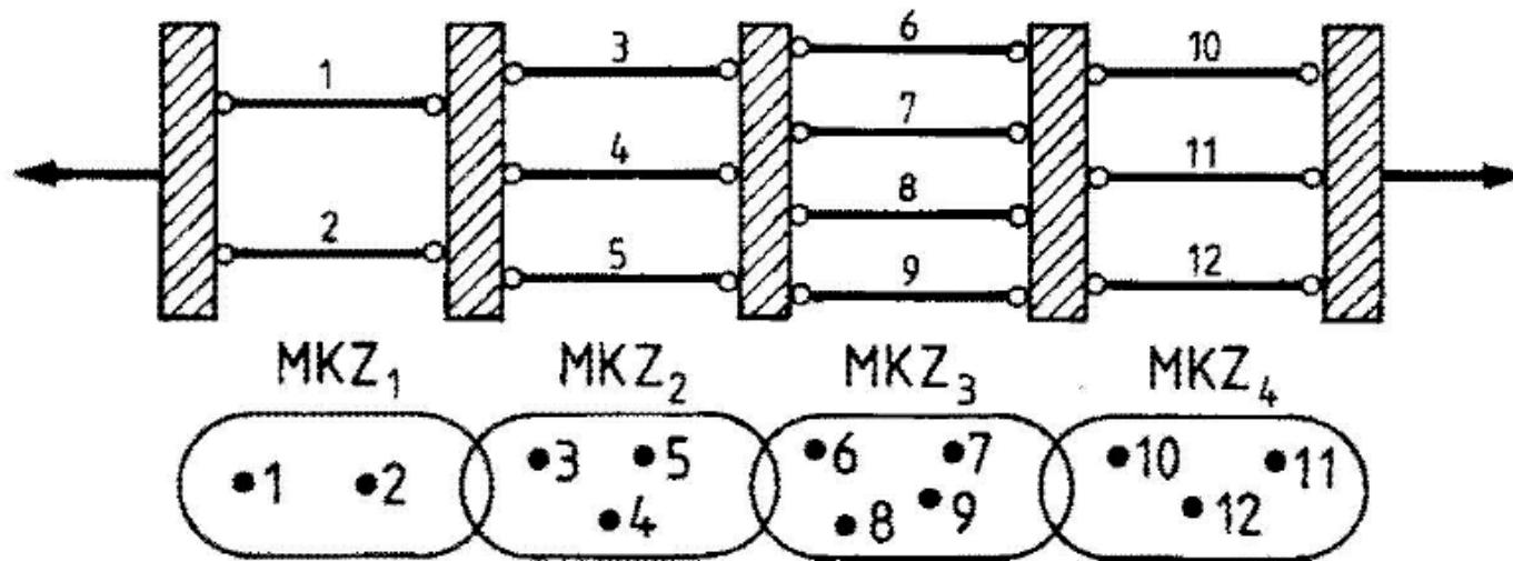
A chain (series system) whose links are bundles of elements (parallel), all decisive elements in a single mechanism are parallel.
