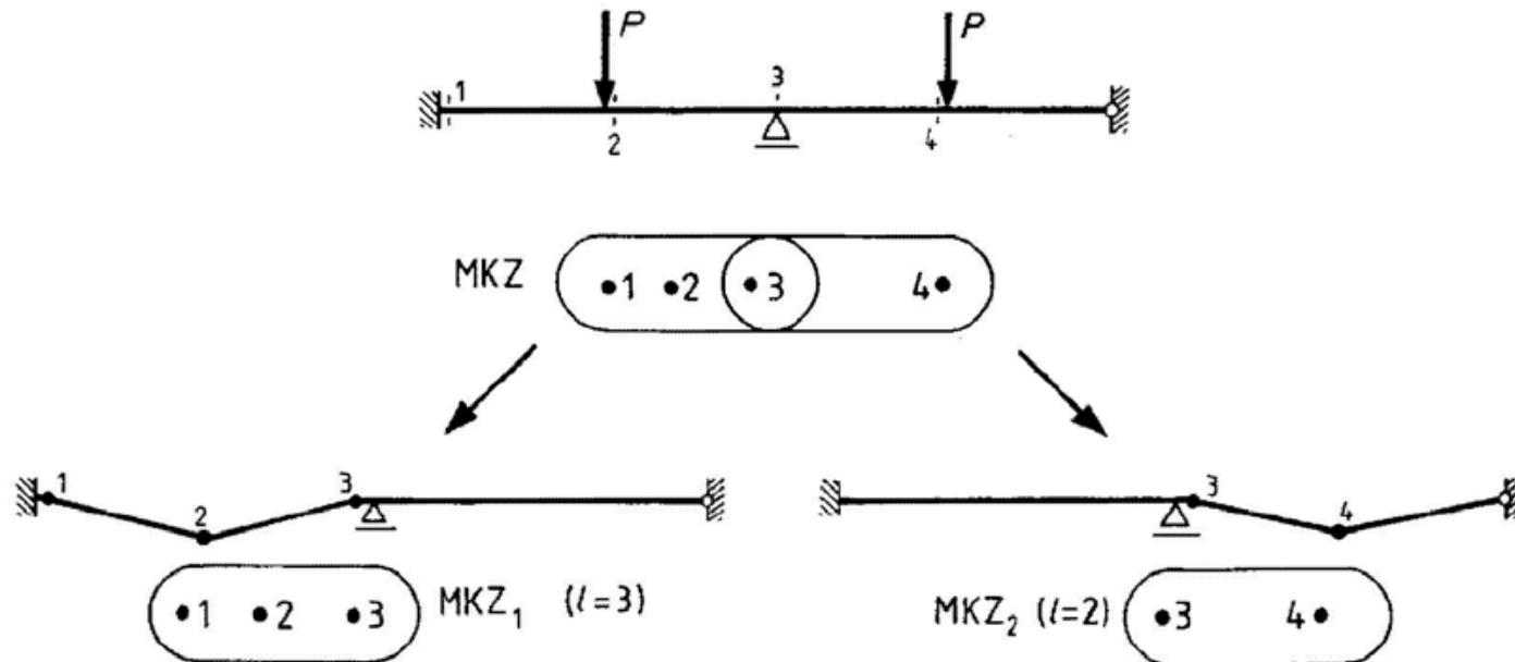
A continuous beam exhibits the following mechanisms - MKZ1 (critical set 1) involving elements (hinges) 1, 2 i 3; - MKZ2 (critical set 2) involving elements (hinges) 3, 4. Both mechanisms MKZ1 and MKZ2 include a common decisive element – a hinge at the middle support (element 3).
