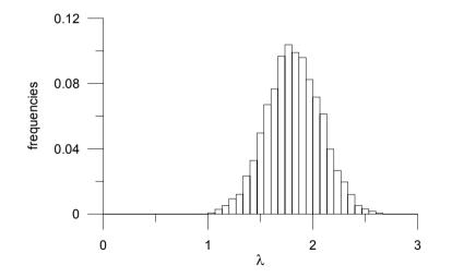
Histogram of the limit state involving the wind load
