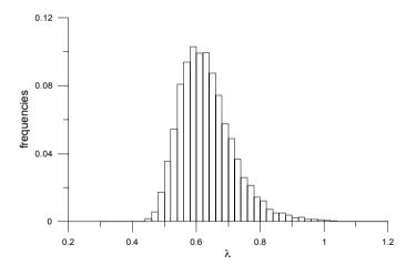
Histogram of the limit state with respect to the yield stress of steel
