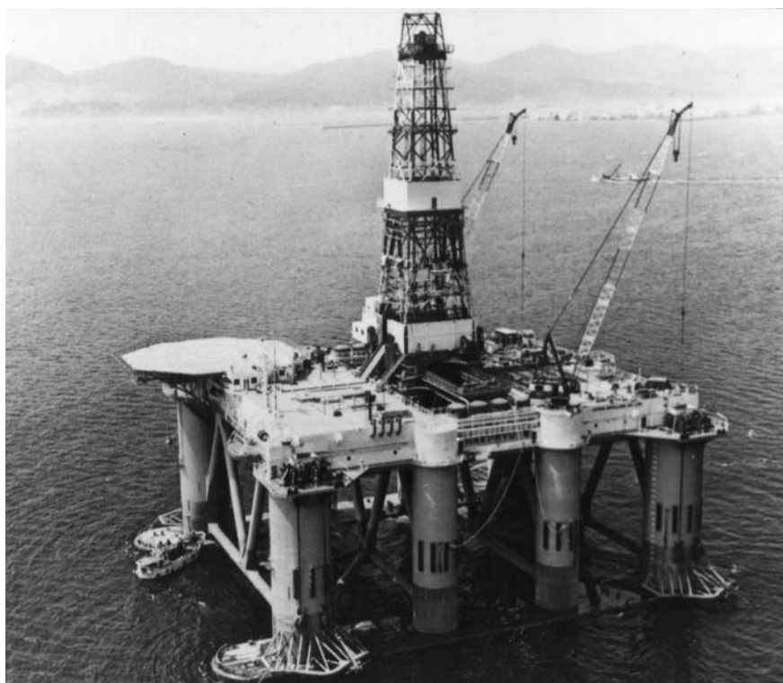
Figure 1.5 A semisubmersible platform (courtesy of the builder, Mitsubishi, Ltd., Tokyo and the owner, Japan Drilling Co.).
