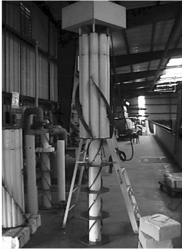
Fig. 1-24. The first Cell Spar had a single lower column (Courtesy of Technip USA, Inc.)
